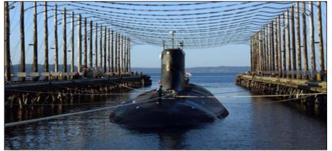
Fig. 1 Demagnetization of the warship
